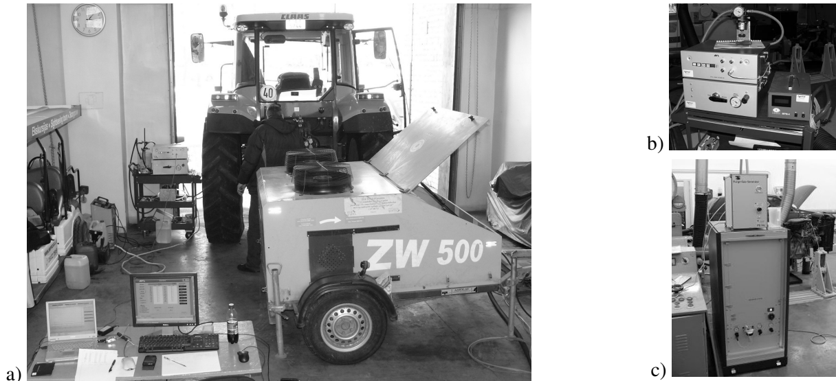
Fig. 1. Test object and measuring equipment: a – CLAAS ARES 557ATX and MAHA ZW-500 ; b – AVL KMA MOBILE ; c – AVL SESAM FTIR
