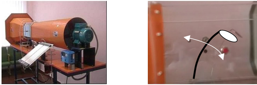
Fig. 19. Wind tunnel and vibrating system inside (right) with console spring and plane lamina
