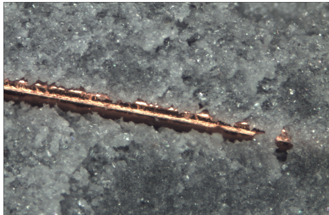
Fig. 6. Cohesion surface failure and distance wire after the perfect curing
