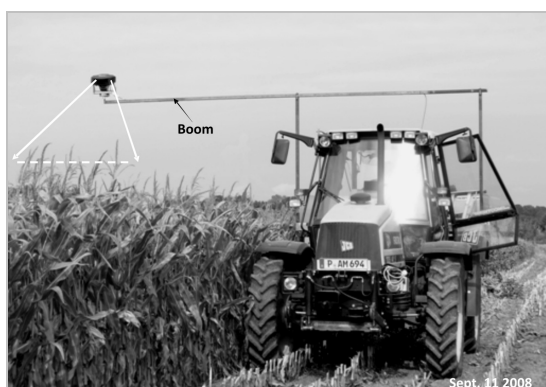
Fig. 4. Test setup for measuring crop biomass in maize
