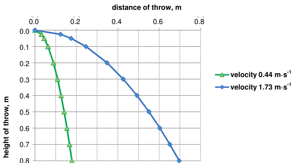
Fig. 5. Calculated trajectories of horizontal throw for velocities
