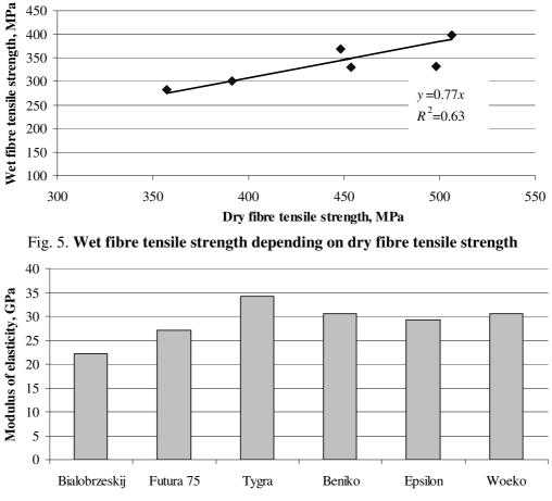
Fig. 6. Modulus of elasticity for different varieties of hemp
