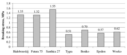
Fig. 8. Lateral compressive strength of hemp stems depending on hemp varieties
