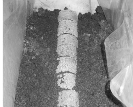
Fig. 2. Briquettes in a flower box ready for “sorption of water by briquettes in soil”
