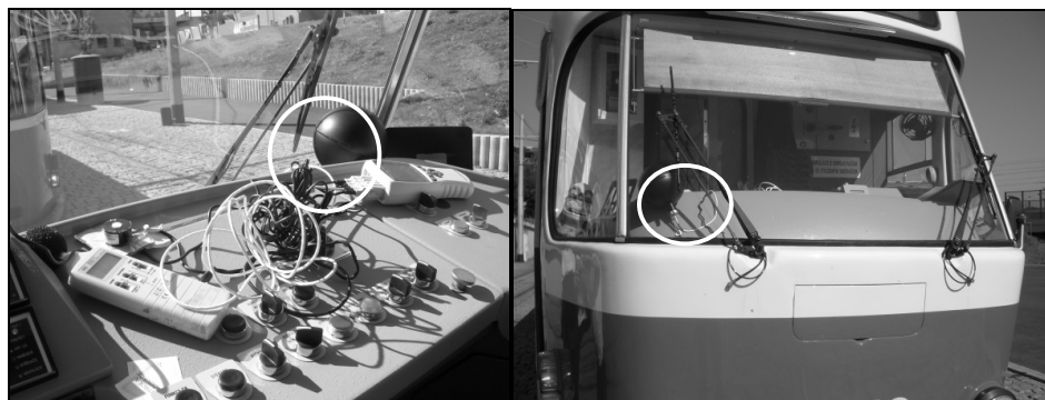
Fig. 2. Measuring devices situated in tram T3 driver’s cabin
