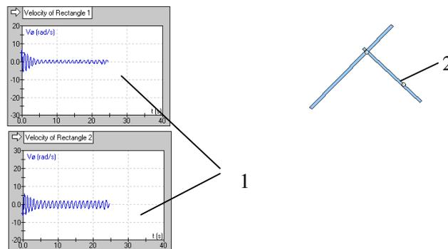
**Fig. 7. Bifurcation of vibration motion (with small amplitude):** 1 – angular velocities; 2 – initial position of double pendulum
