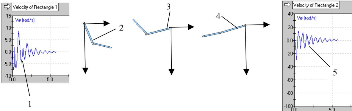
**Fig. 5. Transitional damped vibration motion of pendulum:** 1 – angular velocity of first plate 1 as time function; 2 – initial position of double pendulum; 3 – middle position of pendulum; 4 – close end rest position of pendulum; 5 – angular velocity of second plate 2 (see Fig. 2)
