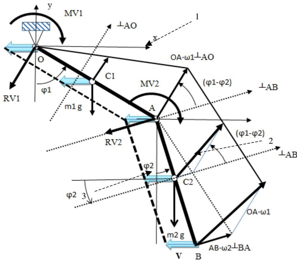
Fig. 3. Graphics of double pendulum points velocities components: 1 – graphic of first pendulum rotation velocity component; 2 – second pendulum relative rotation velocity component; 3 – horizontal flow component;  $RV_1, RV_2$  – principal vectors;  $MV_1, MV_2$  – principal moments
