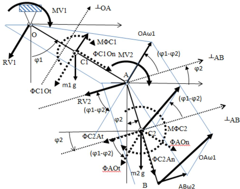
Fig. 4. **D'Alembert's principle forces:** ( $m1g, m2g, RV1, RV2, MV1, MV2$ ) – active forces and their moments;  $\phi, M\phi$  – components of forces of inertia and their moments
