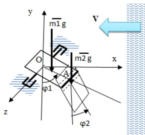
Fig. 1. Double pendulum in fluid flow: 1 – double pendulum; 2 – horizontally flow
