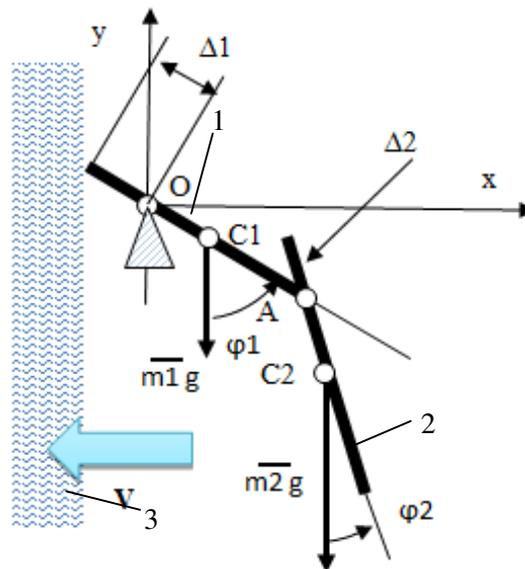
Fig. 2. **Plane model of pendulum:** 1 – pendulum rotating part; 2 – pendulum plane motion part; 3 – horizontal flow;  $\varphi_1, \varphi_2$  – generalized coordinates
