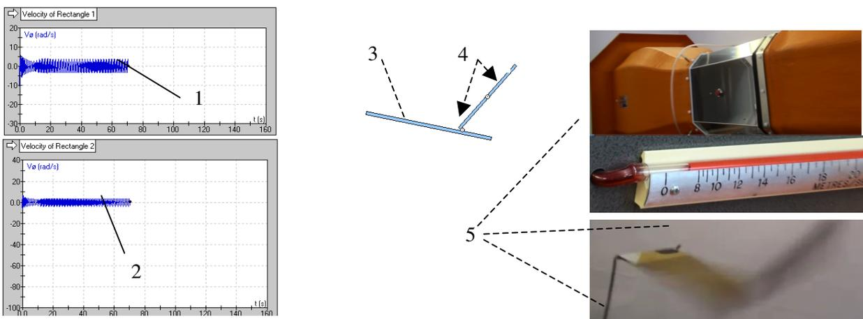
**Fig. 6. Stationary vibration motion of pendulum with large amplitude:** 1 – angular velocity of first plate 1 as time function; 2 – angular velocity of second plate 2 as time function; 3 – initial position of double pendulum; 4 – positions of rotation axis are with eccentricities  $\Delta_1$  and  $\Delta_2$  (see Fig. 2); 5 – experiment in wind tunnel with flow velocity about  $6 \text{ m}\cdot\text{sec}^{-1}$
