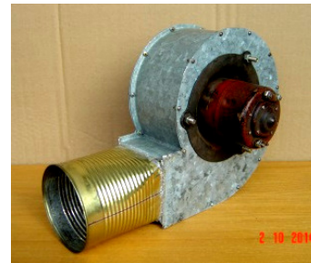
Fig. 3. Centrifugal ventilator with direct current electric motor: 12 V; 4.5 A
