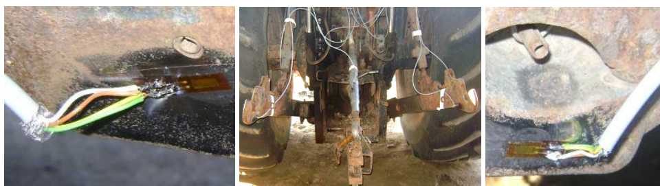
Fig. 2. Strain gauges glued on the tractor rods
