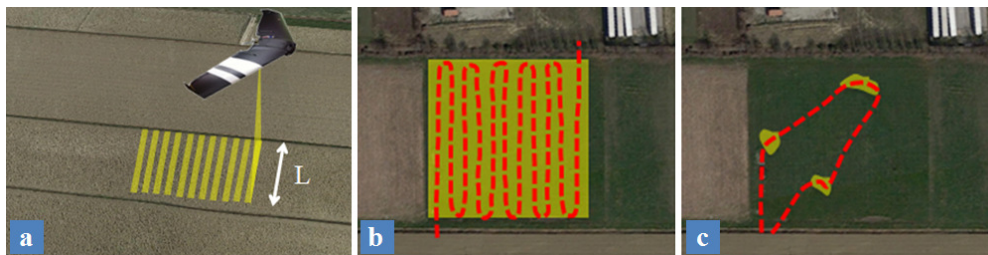
Fig. 6. (a) Dominated width L by UAV on-board sensor or delivery apparatus; (b) raster and (c) point to point strategies in UAVs missions
