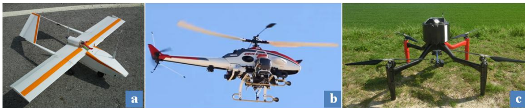
Fig. 2. Three examples of UAVs: a – fixed wing; b – helicopter; c – quadrotor
