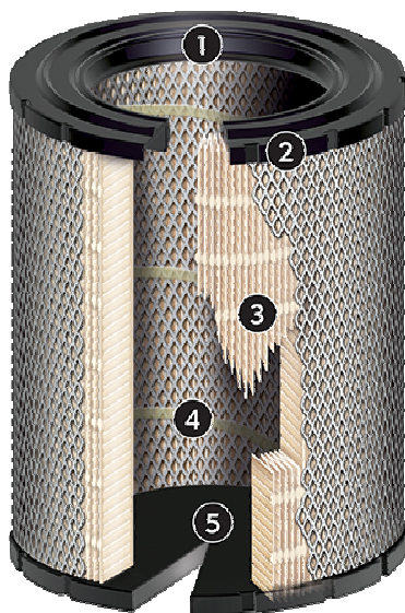
Fig. 1. Air filter construction [1]: 1 – radial seal gasket; 2 – flexible outer edges; 3 – filtering material; 4 – inner liner; 5 – end cap
