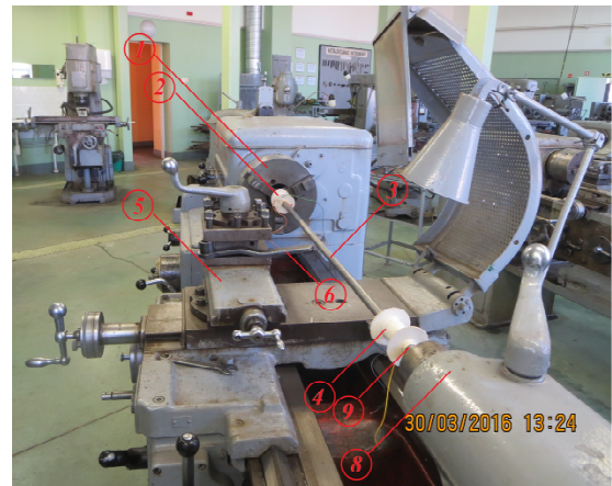
Fig. 6. Scheme of the experiment: 1 – spindle; 2 – magnetization coil; 3 – rod; 4 – receiving coil; 5 – direction of traverse; 6 – stop; 7 – lever; 8 – end head; 9 – rotating center
