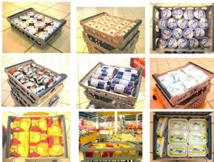
Fig. 4. Secondary package (size 400X300X115 mm) filled by various perishable goods
