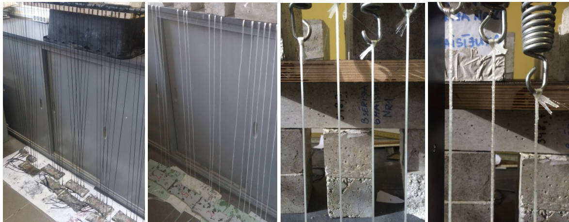
Fig. 1. Composite macrofiber manufacturing: Epoxy matrix/Carbon fiber 1 (CF1), Epoxy matrix/Glass fiber 1 (GF1), Epoxy matrix/Glass fiber 2 (GF2) and Epoxy matrix/Glass fiber 3 (GF3)
