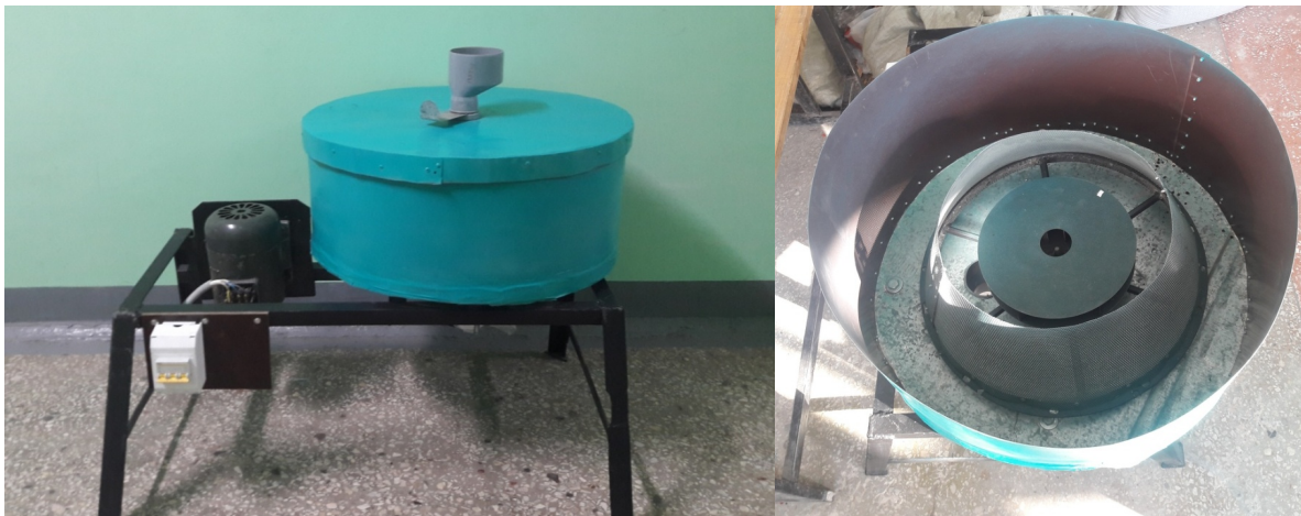
Fig. 2. General view of the peeling machine with the variable deck
