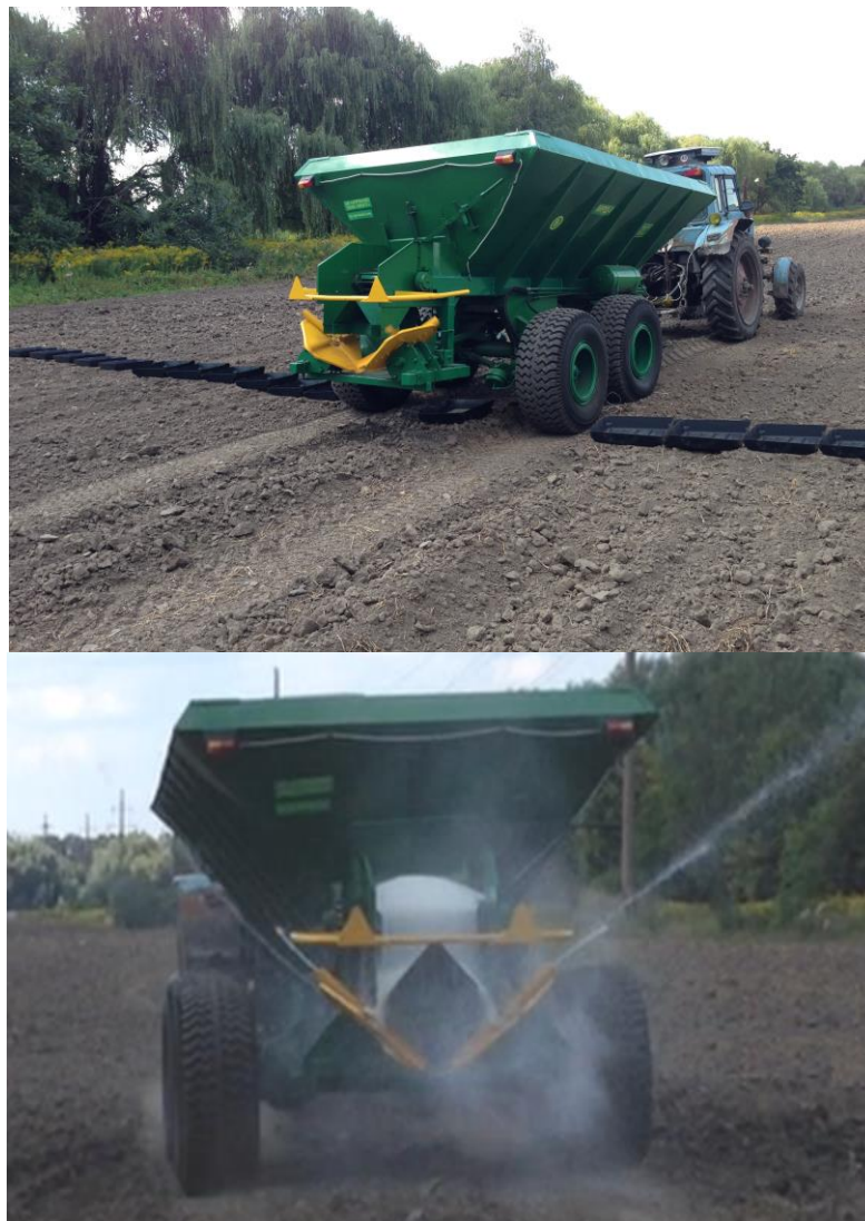
Fig. 1. Experimental equipment for study of the spread of ammonium nitrate by an inclined disk
