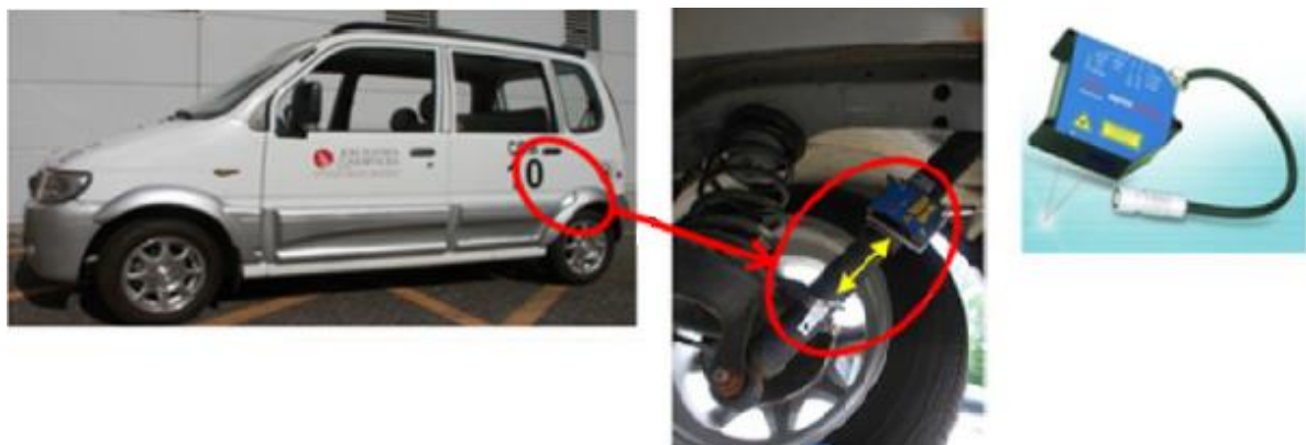
Fig. 5. Place of installation of the energy harvesting shock absorber [57]
