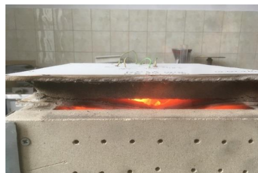
Fig. 12. Equipment for determining temperature dependency on x at fixed time t
