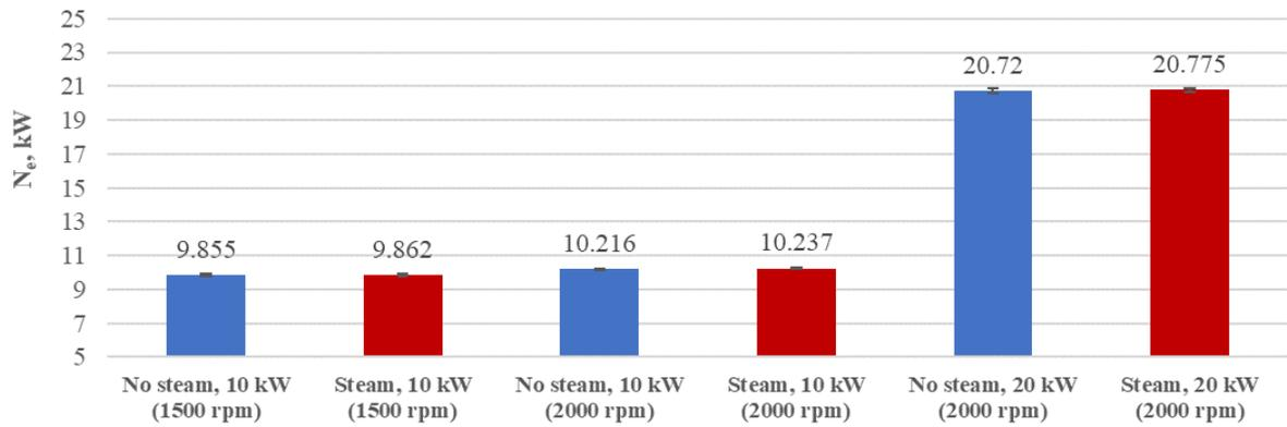
Fig. 5. Power at different testing conditions with and without steam addition
