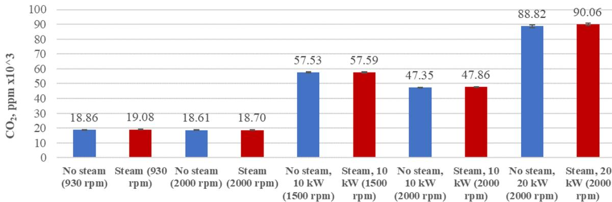
Fig. 3. CO<sub>2</sub> at different testing conditions with and without steam addition
