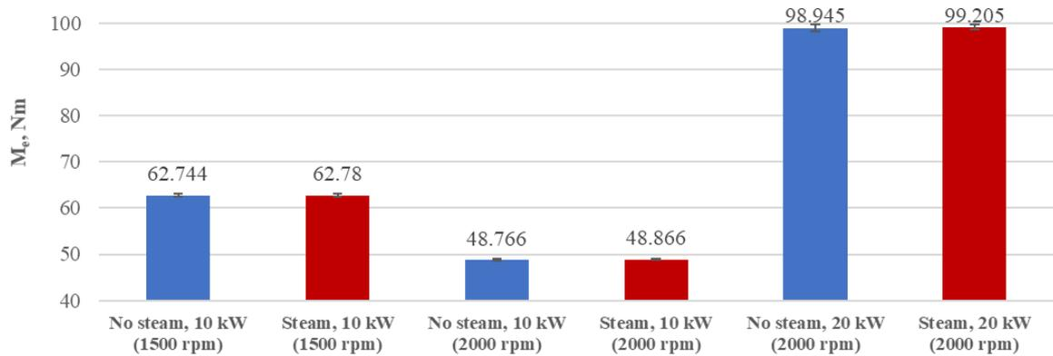
Fig. 6. Torque at different testing conditions with and without steam addition
