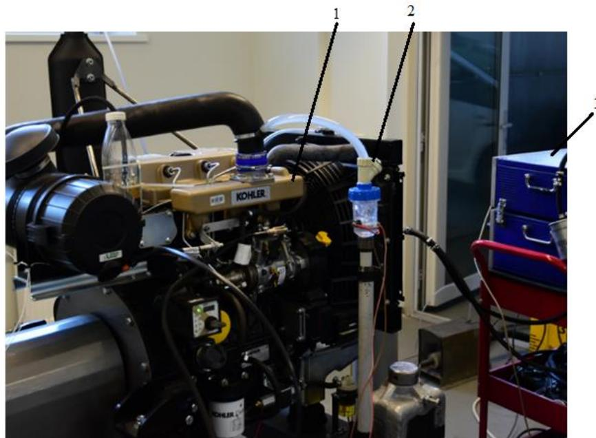
Fig. 1. **Test engine:** 1 – engine; 2 – steam generator;
