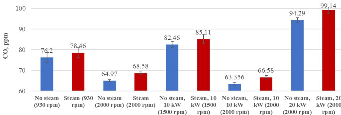
Fig. 4. CO at different testing conditions with and without steam addition
