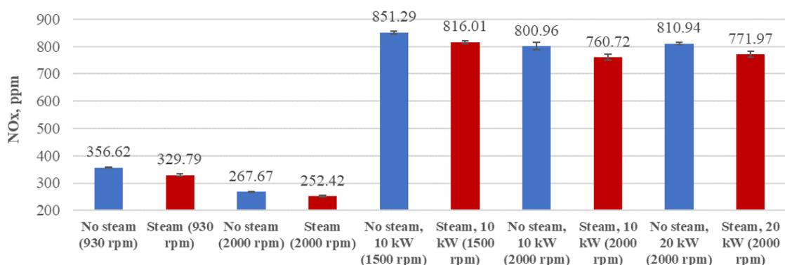
Fig. 2. **NO<sub>x</sub> at different testing conditions with and without steam addition**
