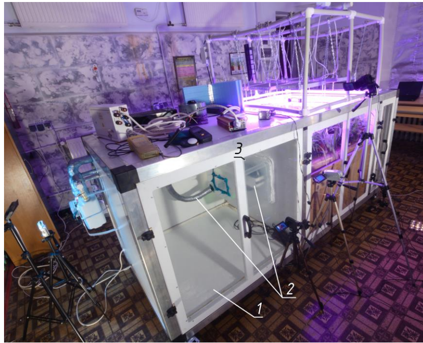
Fig. 2. Gas exchange camera in Laboratory of Heat-Mass Exchange in Green Structures with the tightness monitoring camera, general view (pos. – see Fig. 1)
