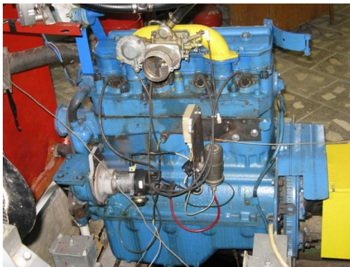
Fig. 1. Gas engine converted from diesel D-243 on a test stand
