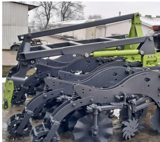
Fig. 1. Fragment of a set for growing and strip sowing of hemp without seeding mechanisms, constructed at Roltex, fot.Roltex [26]
