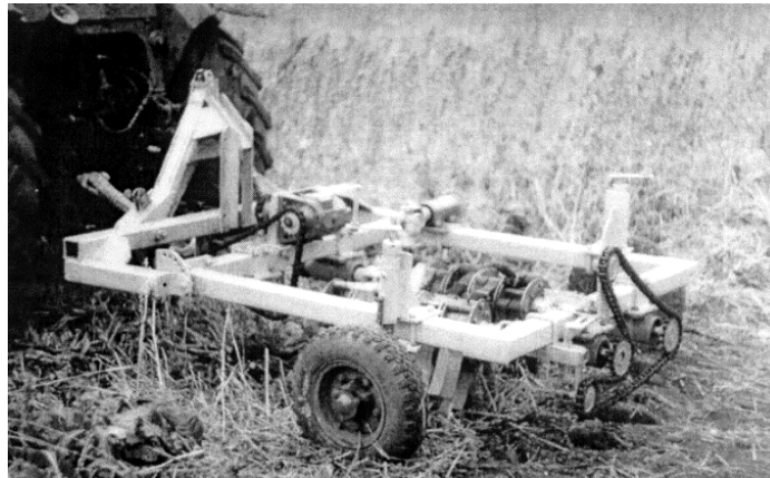
Fig. 1. Two-shaft cleaner of carrot heads from the remaining tops without extracting the heads from the soil
